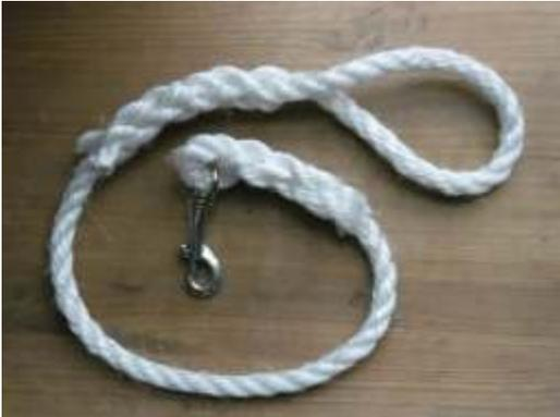
An eye splice at each end of this piece of rope produces a practical dog lead.
